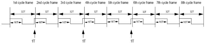
(narrow pulse inserted by BRM0[2:0] setting, here BRM0[2:0]=3)
