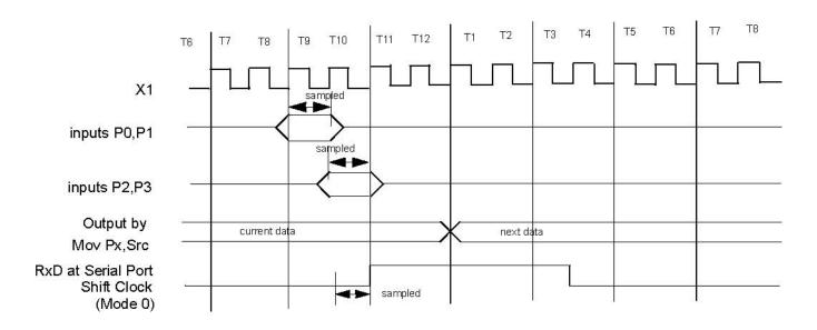
Timing Critical, Requirement of External Clock (Vss=0.0V is assumed)
