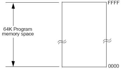
Note: The single flash block address structure for doing as well as program ROM flash.
