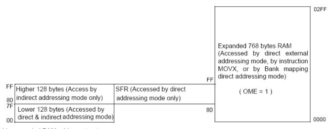
On-chip expanded RAM address structure.
